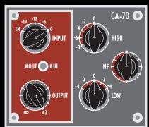
The NF, Hi, and LOW controls all interact to create a unique tone-shaping circuit.
