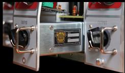
The OUTPUT control trims the gain between the first and second tube stages. This allows you to get your final level set without any tone degradation. It also offers further tone shaping through manipulation of the two-stage EF86 gain structure. With up to 60db of gain available, the CA-286 Amplifier has enough power to boost almost any signal to proper recording levels.
