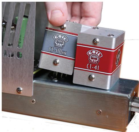
Before inserting modules into the rack tray, make sure both your input and output transformers are firmly seated into the module body. Never plug or unplug transformers while the module is plugged in and powered on.
